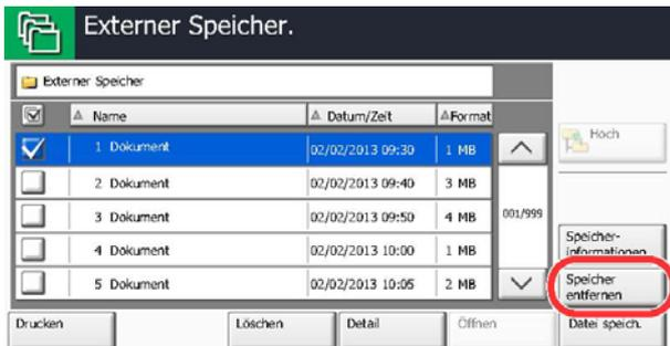
Press [OK], and remove the USB memory after "Removable Memory can be safely removed." is displayed.
